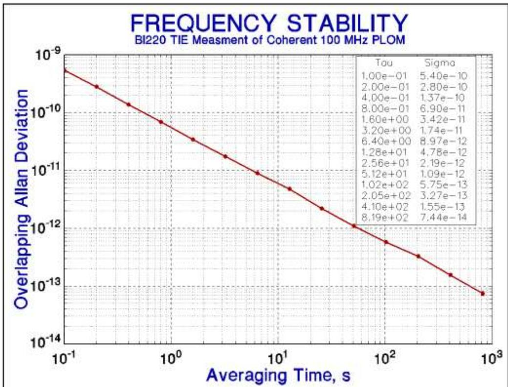
Figure 6. Frequency Stability:  $5.5 \times 10^{-11}$  1-Second White PM Instrument Noise Floor
