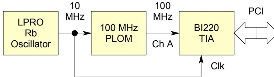
Figure 1. Test Setup – Coherent 100 MHz Phase-Locked Oscillator Multiplier
